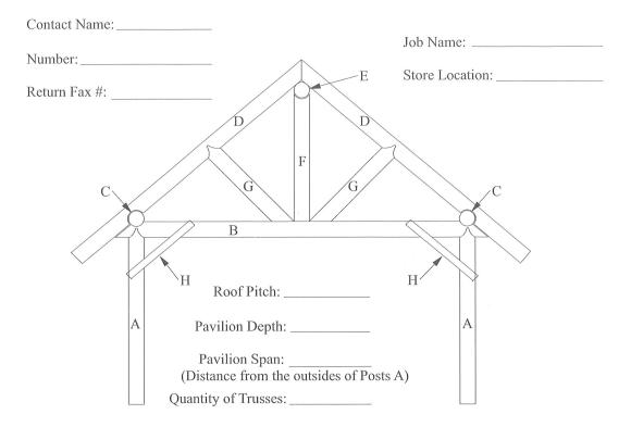
IMPORTANT NOTES: Trusses are not assembled. Site cutting/notching and assembly are necessary. Fasteners not included. Materials only, contractor needs to verify material list, log lengths, and check local codes. Log Supports for header are recommended every twelve feet. No logs available over 24'. Extended lead time necessary for 20' 22' and 24' long logs.
